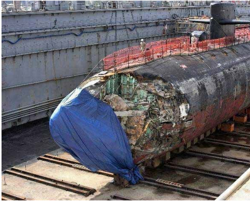
Figure 21.1 Many seamounts remain uncharted. On January 8th 2005, the US nuclear submarine San Francisco en route to Brisbane Australia for a port visit, ran into an underwater mountain at 35 knots about 350 miles south of Guam leaving one sailor dead: a number of sailors were awarded medals for bravery in dealing with over 70 wounded. The seamount is now named the “San Francisco seamount”.
